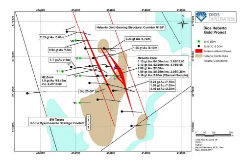
AU33 <u>HEBERTO GOLD</u> 2017 drilling results from gold-bearing hydrothermal altered shears
