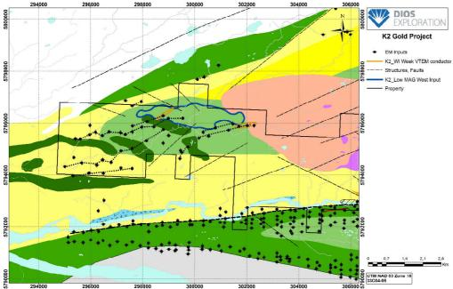
**K2** Farwest inputs and weak VTEM conductors at low magnetic contact New gold occurrence discovered, up to 6.72 g/t gold in rocks and 0.233 g/t gold in soils
